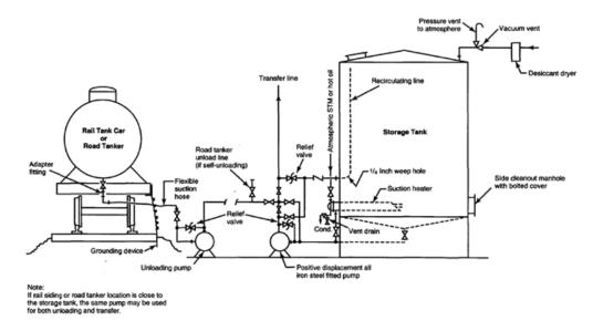
Figure 10-1 Typical Tank Car Unloading and Storage System
